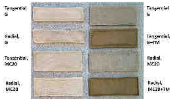
Examples of the cross-section of aspen (left) and birch (right) board, with 30% and 10% target degree of compression, respectively. Figure: Veikko Möttönen
